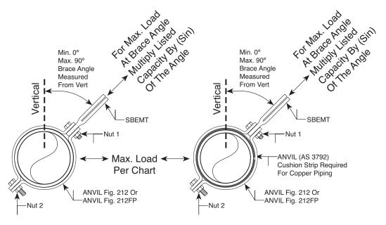
NOTES: Capacity based on seismic testing considering both tension and compression. To convert listed horizontal capacity to angle capacity multiply listed capacity by (sin) of the angle.
