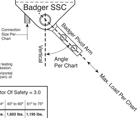
Capacity of bracket based on seismic testing considering both tension and compression.
