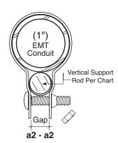
Tighten Torque-Off Hex Nut Until Hex Head Breaks Away. Gap And Bolt End Deformation May Vary Other Than Depicted Due To EMT Conduit Member And Vertical Support Rod Size Combinations
