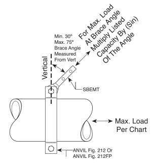
NOTES: Capacity based on seismic testing considering both tension and compression. To convert listed horizontal capacity to angle capacity multiply listed capacity by (sin) of the angle.
